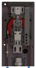
The enlarged guide wheel (red on the left) adopts a center design, occupying the entire U-shaped arc surface, and drives the feeding and discharging at the same time to prevent the jamming of the material belt.
