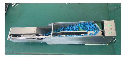
**Principle:** Through the components selection track, NG components through the reflux Belt return: The selected material is transported to the component level by direct vibration
